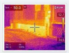
By insulating the interior of your foundation, you will be able to eliminate tremendous amounts of heat loss that can be seen in this IR images from the outside.
