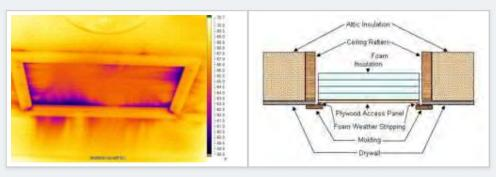
Openings used for access to the attic such as hatches and scuttles, doors into knee walls, and drop-down stairs should be air sealed and insulated.
